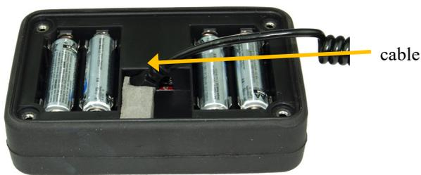
Figure 1. Sensor cable plugged into jack
