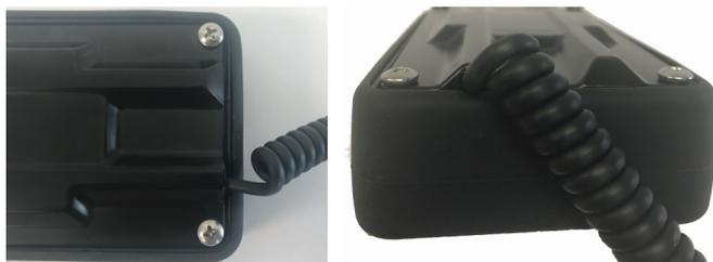
Figure 2. Sensor cable fed through slot
