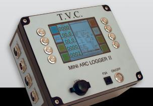
Its 5.7-inch TFT screen provides a clear view of all monitored welding parameters and the sealed battery allows up to eight hours of monitoring time between charge cycles.
