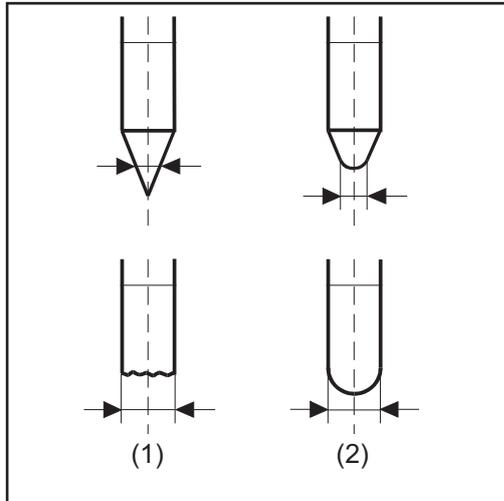
On MagicWave power sources, an automatic cap-shaping function is available for the TIG AC welding process:
