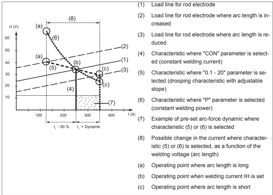
The characteristics (4), (5) and (6) shown here apply when using a rod electrode whose characteristic corresponds - at a given arc length - to the load line (1).
